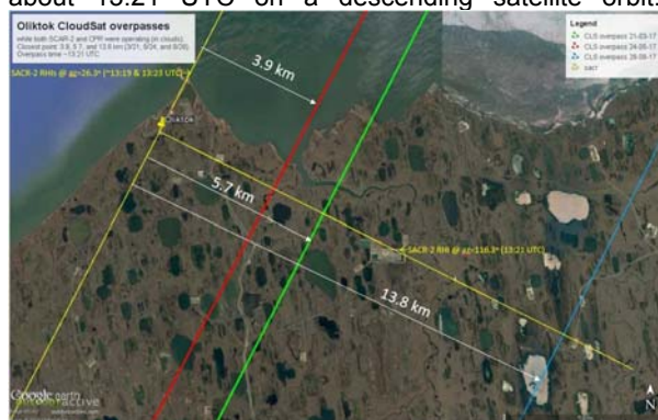
FIG.1. Center beam CPR ground tracks during the overpasses on 21 March (green), 24 May (red) and 28 August (blue). Yellow lines show SACR RHIs parallel and perpendicular to the CloudSat ground tracks. Distances from the AMF3 and the center of the CPR footprint are in white.
