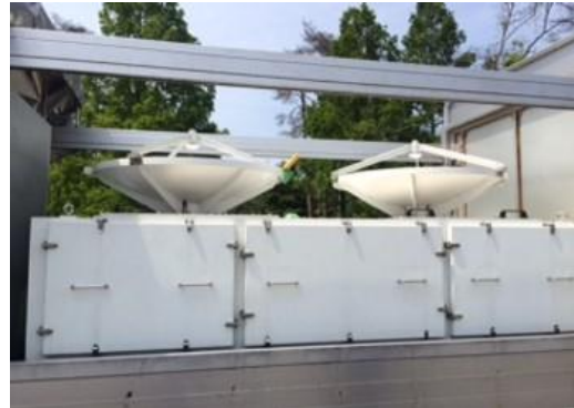
Figure 2. Cloud Profiling Doppler Radar FALCON-I. It consists of two 1-m diameter antennas.
